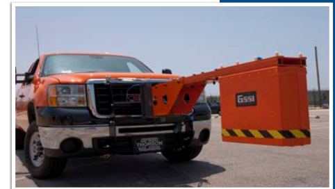
Vehicle-mounted RoadScan system integrated with FWD.
