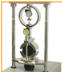
Marshall test in the analogical mode.
