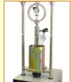
CBR test in the analogical mode.
