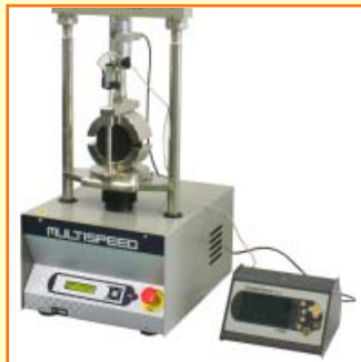
Marshall test in the digital mode.
