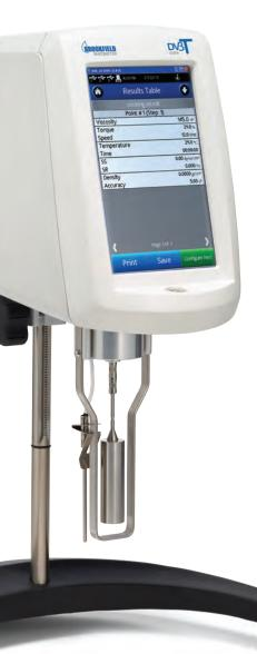
**Integrated Temperature Control** with connection to Brookfield TC series Baths and AP controller or Brookfield Thermosel System.
